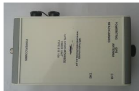
GPS Synchronized Timer Unit Type 818 100
