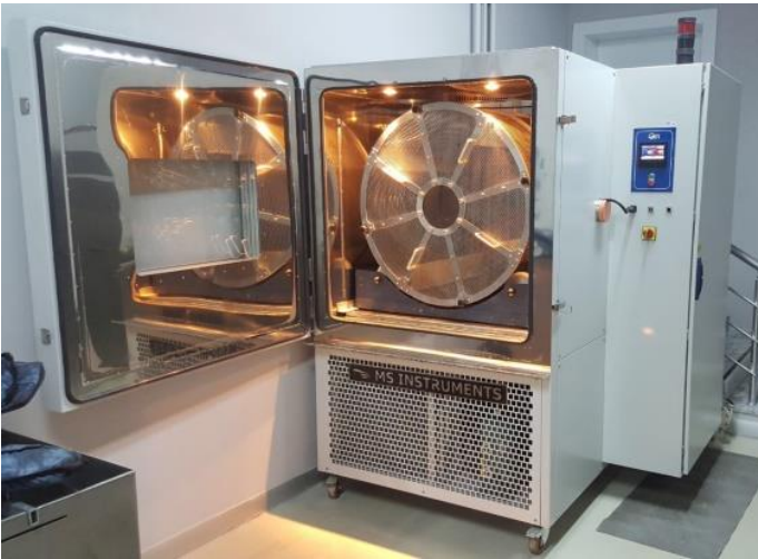
CONDITIONING CHAMBER SHOWING TUMBLER (NIJ 0101.06)
