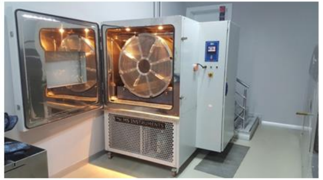
Conditioning Chamber showing tumbler
