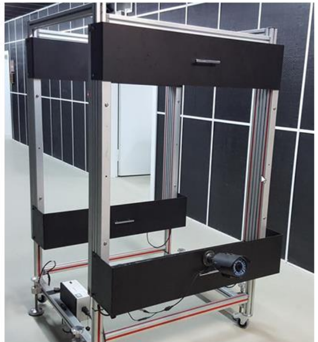
Velocity system rear view (showing target CCTV camera)
