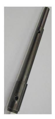
For ammunition proofing, a standard range of test barrels is normally specified. This is to ensure that the impact of the test environment on the ammunition under test is negligible.
